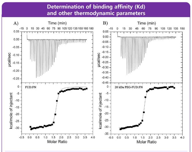
Determination of binding affinity (Kd) and other thermodynamic parameters using Isothermal Titration Calorimetry (ITC). All experiments were performed using pH 7.4 PBS, 25°C chamber conditions, and human plasma FN. A) FUD into FN and B) 20 kDa PEG-FUD into FN experiment sample isotherm and thermograph. Each experiment was repeated in triplicates.
